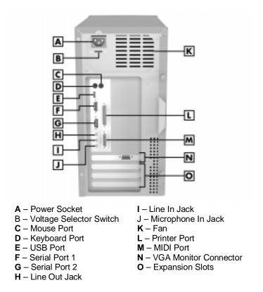
External connectors allow the attachment of peripheral devices such as a monitor, keyboard, mouse, and printer. The system has the following external connectors.
